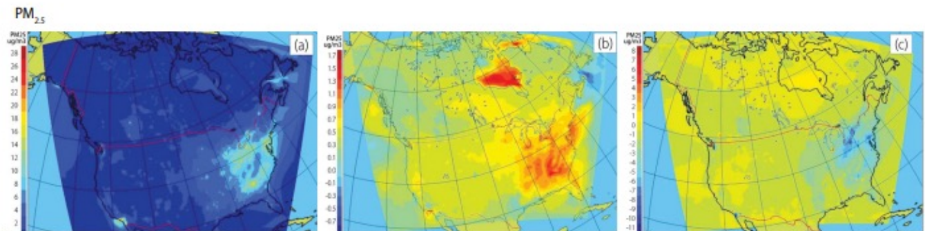
FIGURE 2: a) The ten year average "current" mean summer (June-July-August) 24-hour average PM 2.5 concentration; b) projected changes in the summer 24-hour average PM 2.5 concentration due to climate change with constant air pollutant emissions; and c) projected changes to PM 2.5 for the future with the combined effects of climate change and possible future decreases in air pollutant emissions (Source: Kelly et al., 2012). Note the different contour intervals used in each panel.
