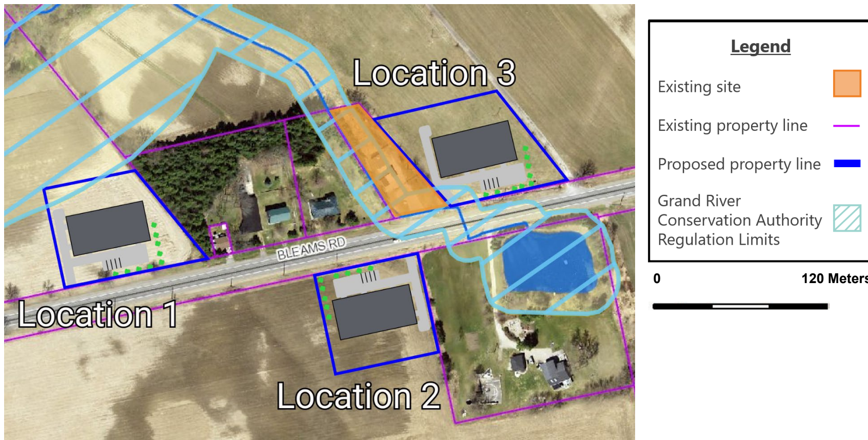
Figure 3.1: Preliminary site location alternatives
