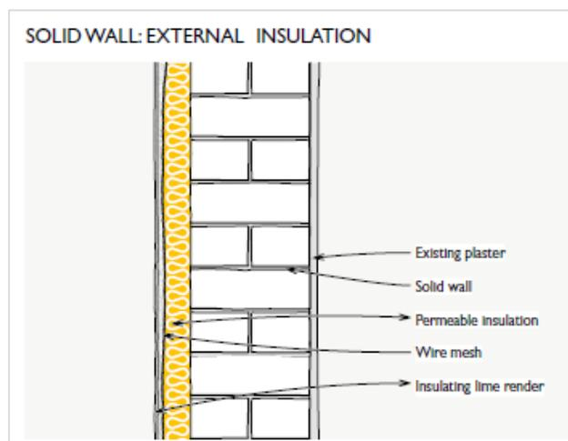
Image: Illustration of the addition of a permeable insulating solution with batts fixed to the masonry and finished with a 'breathable' lime render (English Heritage, 2012, p.14)
