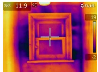
Image: Thermal Imaging of cold air leaking through the window trim (City of Vancouver, 2014, p. 18)
