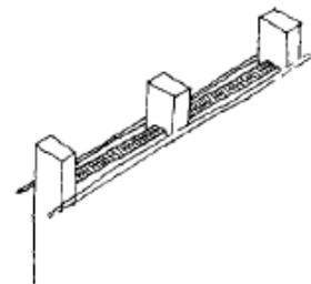
Rigid insulation in wood studs.
