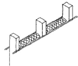
Batt insulation in wood studs.
