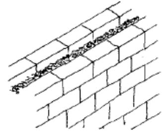
Blown-in insulation in a masonry cavity wall.
