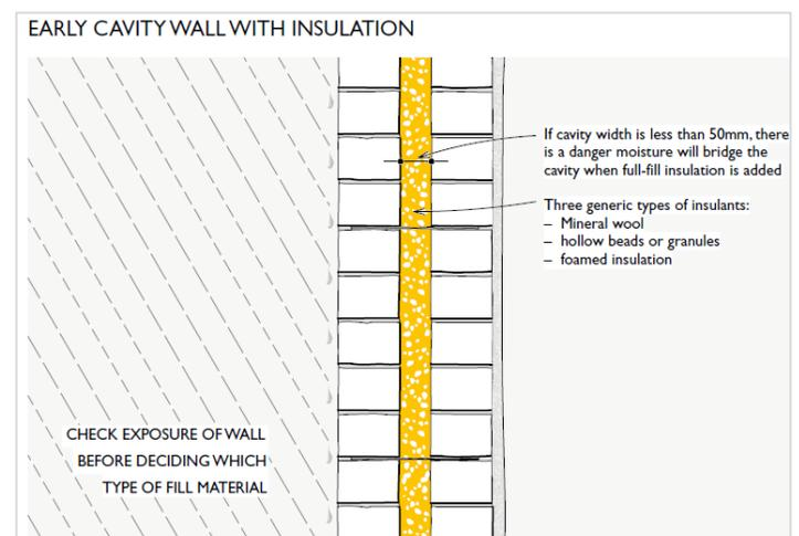
Image: Illustration of an early cavity wall with insulation (English Heritage, 2012, p.15)
