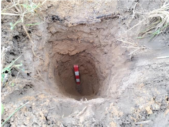
Image 22: Test pit profile demonstrating an absence of A-horizon overlying B-horizon.
