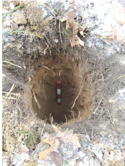
Image 11: Test pit profile demonstrating intact A-horizon overlying B-horizon.
