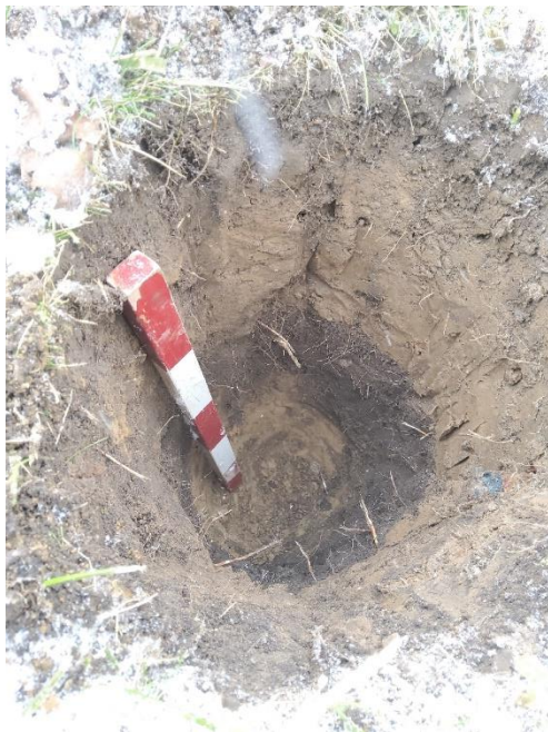
Image 14: Test pit profile demonstrating intact A-horizon overlying B-horizon below laid soils.
