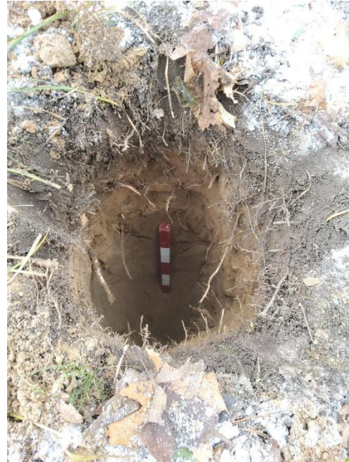
Image 12: Test pit profile demonstrating intact A-horizon overlying B-horizon.
