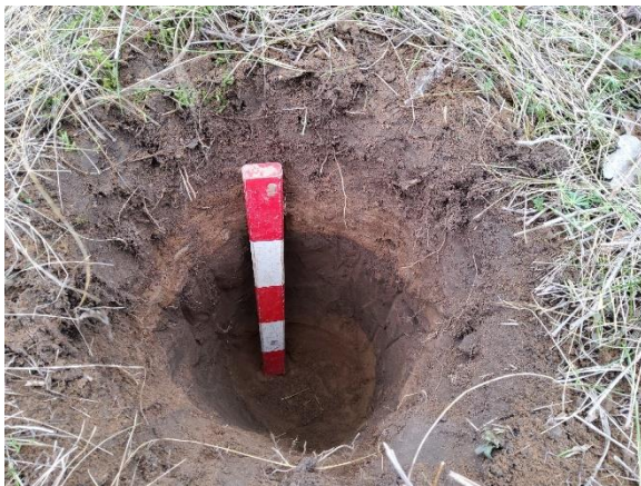
Image 14: Test pit profile demonstrating intact A-horizon overlying B-horizon below laid soils.
