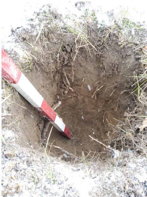
Image 13: Test pit profile demonstrating intact A-horizon overlying B-horizon.
