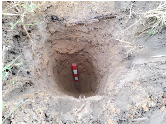
Image 24: Test pit profile demonstrating an absence of A-horizon overlying B-horizon.
