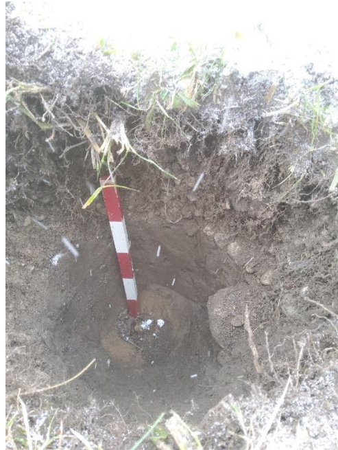
Image 26: Test pit profile demonstrating an absence of A-horizon under fill soils.
