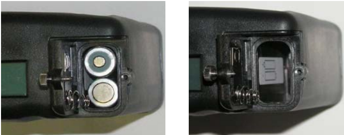
Figure 2. Insertion of Batteries
