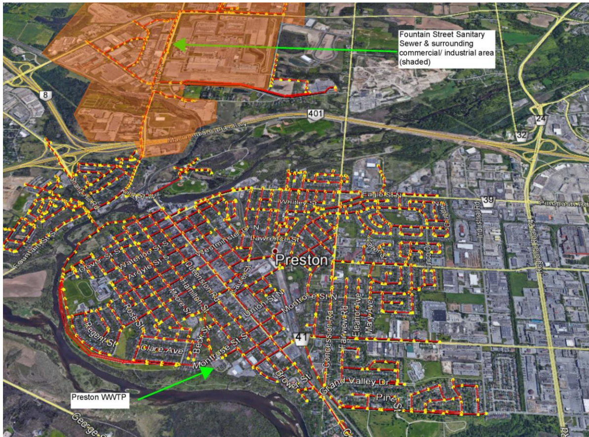
Figure 1 Preston Sanitary Sewer Network
