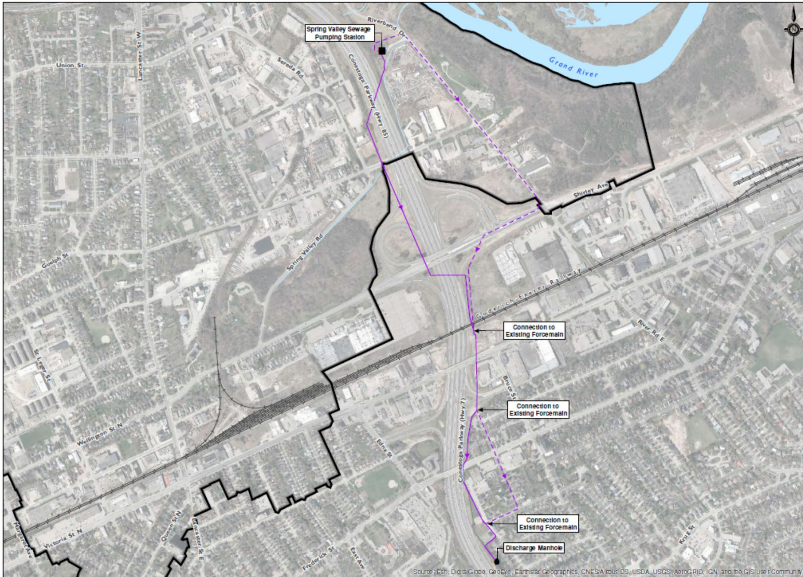
FIGURE 16: EXISTING AND PROPOSED FORCE MAIN
