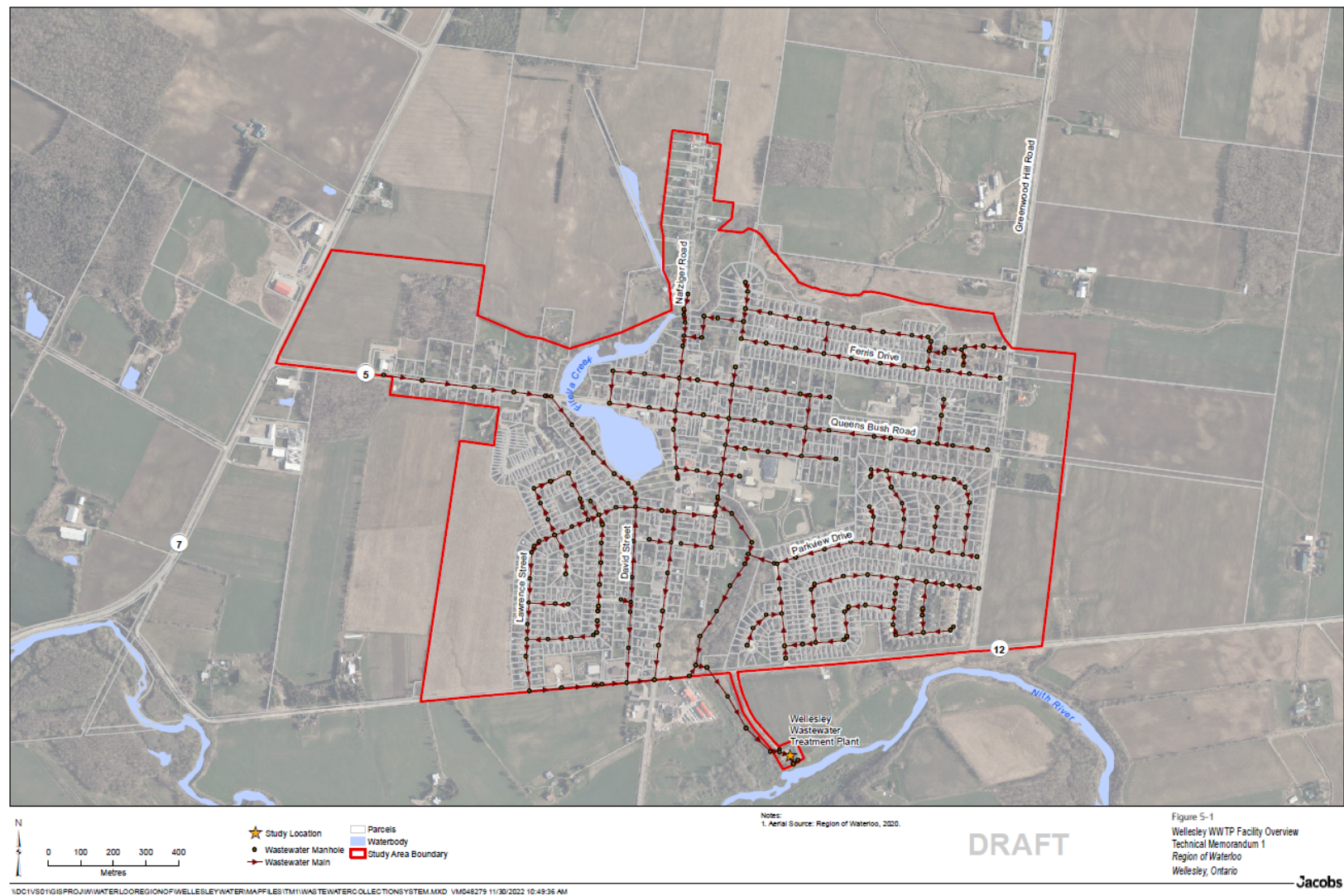
Figure 4-5. Wastewater Collection System Overview
