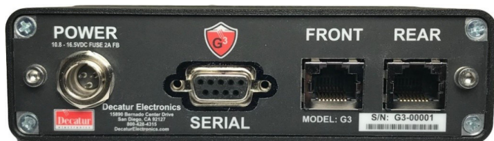
Figure 4b The G3™ rear interface
