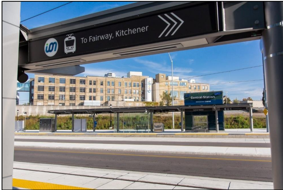
Figure 4-2: Adjacent Side-Loading Platform Configuration
